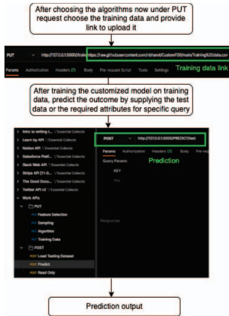
Fig. 2. Demonstration of training and prediction in proposed module
