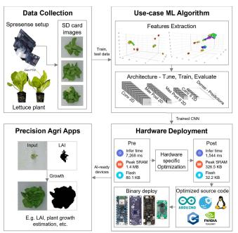
Figure 1: Components, design flow of embedded ML pipeline.
