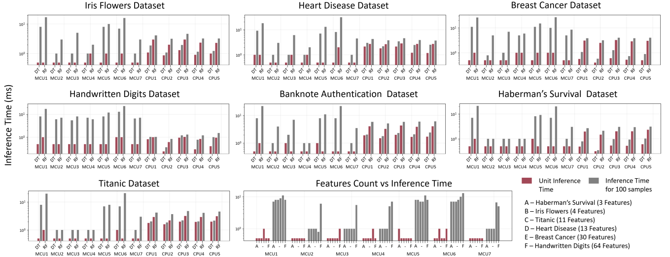
Figure 2: Demo results: comparing the time consumed by MCUs 1-7 (using our implementation) and CPUs 1-5 (using Python scikit-learn) when performing inference for datasets of various feature dimensions (3-64) and class counts (1-10).
