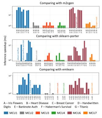
Fig. 2. Comparing inference time for 100 samples: Speedups achieved when porting and executing the models on MCUs using our proposed method.
