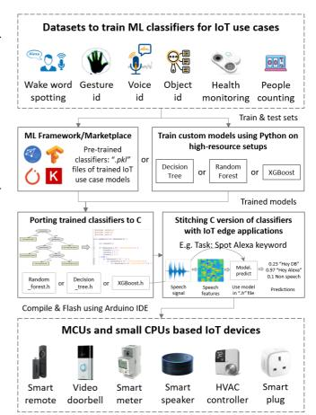
Fig. 1. Design flow to deploy and execute ML models on MCUs of tiny IoT devices: The models ported and stitched using our proposed approach produce ultra-fast classification results while consuming 0 bytes of SRAM.
