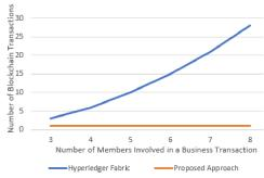
Fig. 5. Compare the number of transactions in the Transaction Flow
