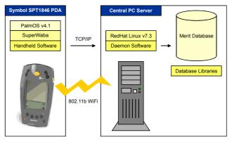
Fig. 1: Hardware and software layers: handheld client, network server and product database.
