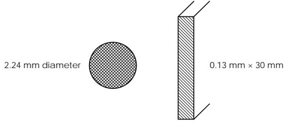
Figure 4: Round versus foil conductor
