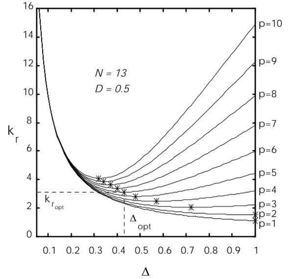
Figure 3: Plot of  $k_r$  versus  $\Delta$  for 13 harmonics and various numbers of layers ( $D = 0.5$ )
