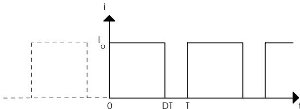
Figure 1: Pulsed current waveform with a duty-cycle of  $D$
