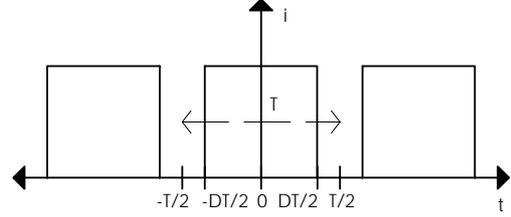
Figure 2: Same waveform taken as an even function
